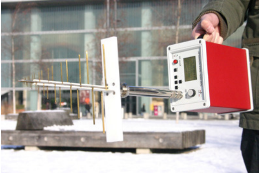
Fig. 5 The mains-free operation provides advantages in field testing such as in-building and outdoor propagation measurements or testing in shielded rooms.
