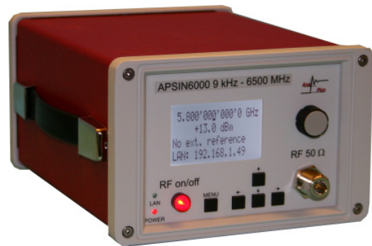
Fig 1 APSIN6000 Front View (WxLxH is only 17 x 22 x 10 cm, weight < 2.5 kgs)
